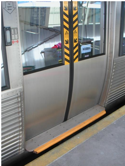
Figure 5 - Westrail EMU doorway with tread buffer strip
