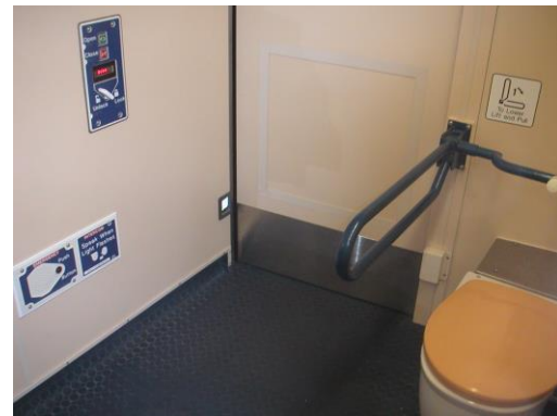
Figure 8 - QR IMU Wheelchair Accessible Toilet
